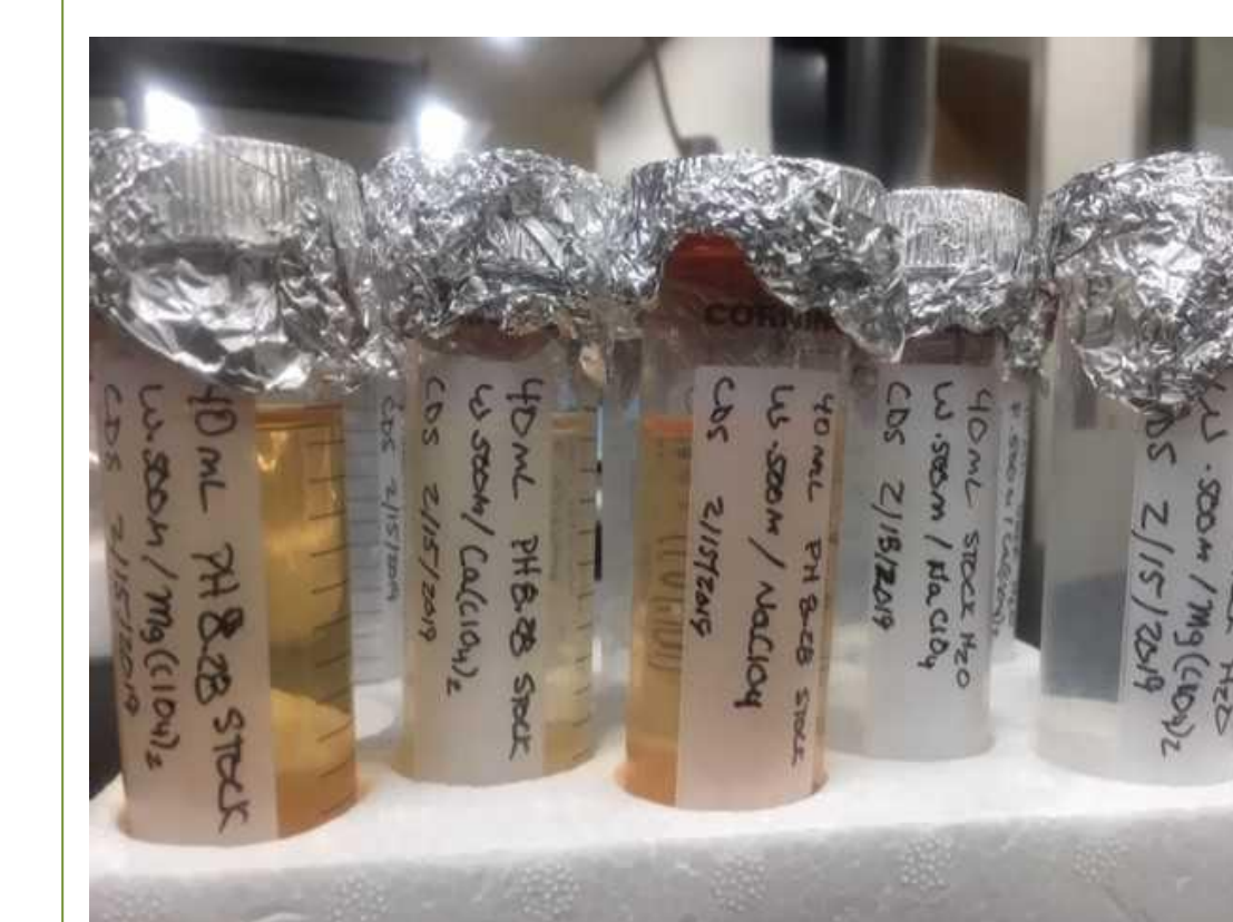
Figure 16: Possible oxidation of Solutions with pH 8.3 and perchlorates
